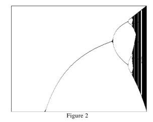
Figure 2 shows a Bifurcation Diagram of the iterative system x(n+1) = k x(n) (1-x(n)). The x axis shows attractors (fixed points) of x for  $n \rightarrow \infty$ . The parameter k is depicted on the y axis.
